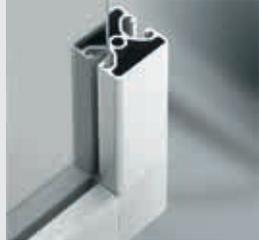
The Clamp-Profile Fastener can be combined with any desired Profiles 6 30x30 or 8 40x40 and also with the existing Clamp Profiles 6 30x30 or 8 40x40. The fact that the Clamp-Profile Fastener has a special cavity means that the panels to be fitted in the profile grooves do not need to be notched.
