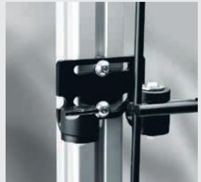
The Dual-Rod Mesh is first hung from a preassembled Dual-Rod Mesh Hanger, and then screwed into position with further Hangers. Recommended spacing of Hangers: 3 section heights, corresponding to 600 mm.
