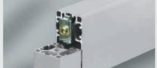
Standard-Fastening Set ESD is used in the same way as a conventional Standard-Fastening Set. The special design of the fastening screw partially destroys the insulating anodized layer on the profile groove and creates an electrical contact between the connected profiles.
